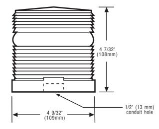
Use Cat. No. GSK-KIT gasket kit for weatherproof surface mount installation on AC units
