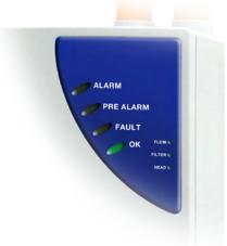
**ALARM** Illuminates to indicate that the smoke level has passed the detector's alarm threshold, and the normally open Fire relay contacts have closed.
